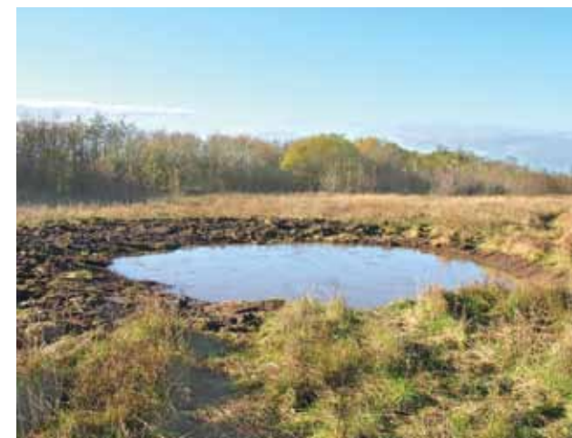
A large test hole allows water levels to be monitored for up to a year, during which it may function as an amphibian breeding pond and should not be filled in. This one is 7 m in diameter and 1.2 m deep (David Orchard)
