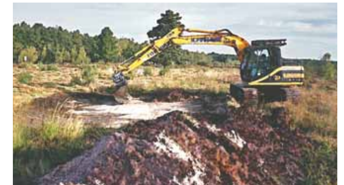
Machinery such as a 13 tonne, tracked, 360° excavator is suitable for creating natterjack scrapes (John Buckley)
